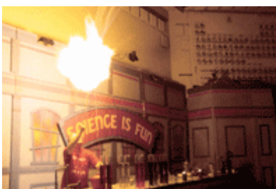
Fig. 6-2: Dr. Shakashiri demonstrates that when the candle is touched to the balloon full of hydrogen and oxygen, a loud explosion will result.
