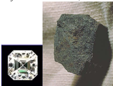
Fig. 1-6. Both diamond and coal are forms of the element carbon, but diamond has a greater density.
